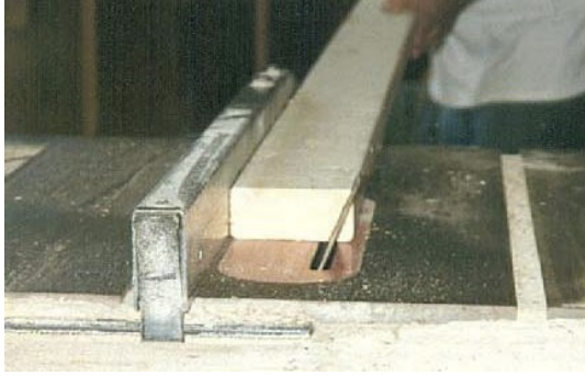
Sawing the beveled overhang (22 1/2 deg)
